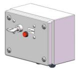
To release the key, an external signal must be received to energize the solenoid. With the solenoid energized the LED will illuminate to confirm that the key can be removed ensuring the power is off
