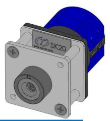
The SK is a key driven electrical switch interlock ideal for the controlled isolation or switching of low current. This product is used to release a key and the switch contacts change to isolate the process. This type of isolator should be used for short term, off load isolation. The unit is ready for mounting into an existing panel or for surface mounting within its own IP65 rated enclosure. The SK is manufactured from either brass or stainless steel.
