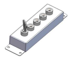
The key exchange box is designed to allow the release of secondary keys by trapping one or more initial keys. The need for this type of product usually arises where there is multiple access to a hazardous area. The key exchange box will be the link between the isolation locks and the access locks to the hazardous area.
