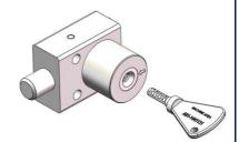
By inserting and turning the key in the bolt interlock, you can retract the bolt, e. g., releasing the disconnector. This will trap the key into the lock.
