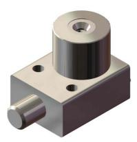
The SD lock is a key operated mechanical bolt interlock that is suitable for the control of electrical switchgear. The standard unit comes with a 16 mm diameter bolt available in various lengths, that is used to control the rotation or movement of operating handles or toggles of electrical switchgear. Many suppliers of switchgear equipment have mounting kits available for ARMADILLO interlocks. The lock is manufactured in brass or stainless steel.
